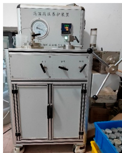
Figure 4. Fluid–rock reactor at high temperature and pressure.
