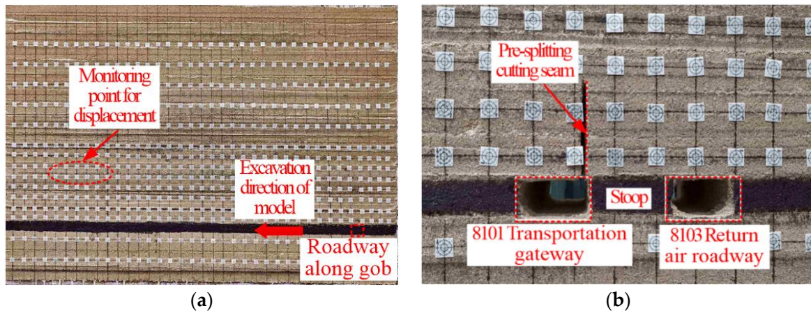
Figure 5. Models before and after roof cutting. (a) Model before roof cutting. (b) Model after roof cutting.
