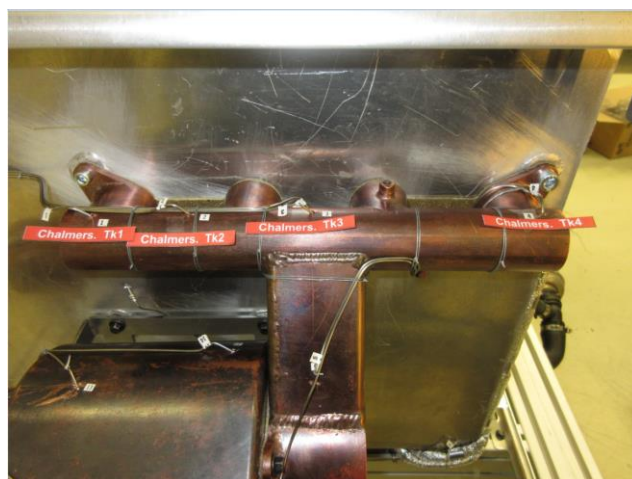
Figure 3. An example of embedded thermocouples installation.
