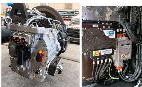
**Figure 9.** The electrical motor and traction inverter.
