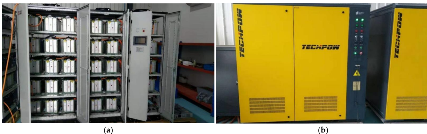
Figure 7. Efficiency test of supercapacitor storage. (a) Supercapacitor storage. (b) Efficiency test equipment.
