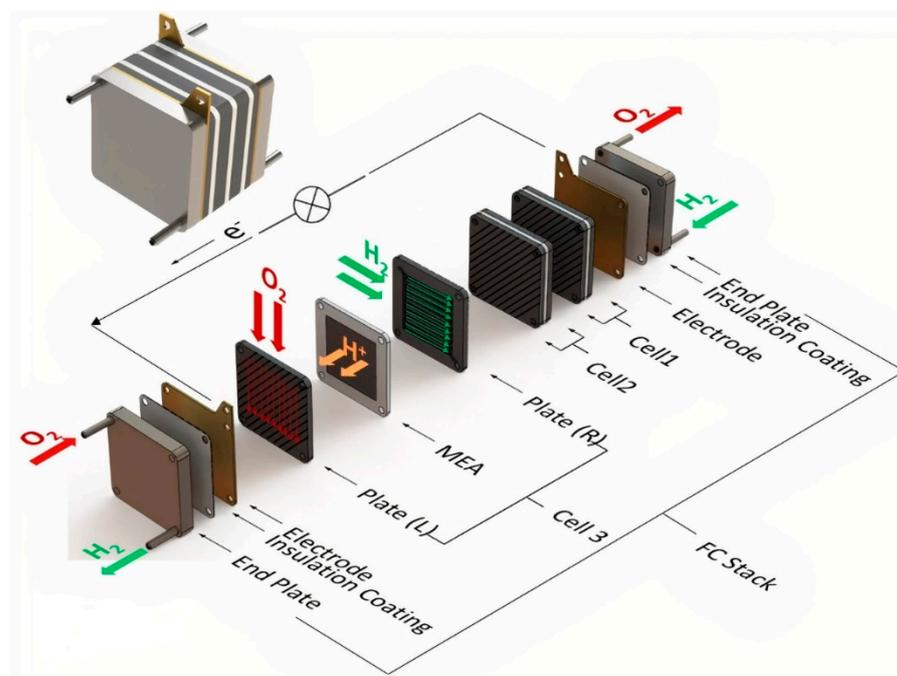
**Figure 7.** Fuel cells stack and components schematic [140]. (With permission, license number: 5430310482582).
