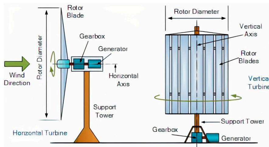
**Figure 3.** Wind turbine types: VAWT and HAWT [66]. (Open Access).
