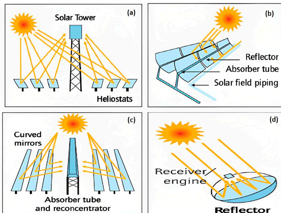
**Figure 1.** Recent available CSP technologies: (a) solar thermal tower, (b) parabolic trough collectors, (c) linear fresnel reflectors, (d) parabolic dish [49]. (Source: International Energy Agency, Technology Roadmap-Concentrating Solar Power).
