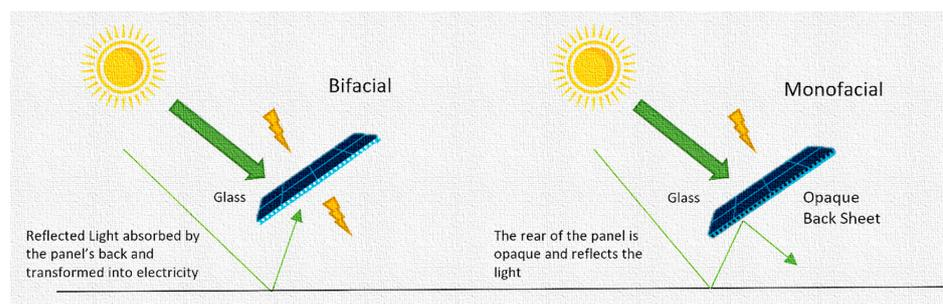
**Figure 2.** Bifacial vs. mono-facial solar panels.
