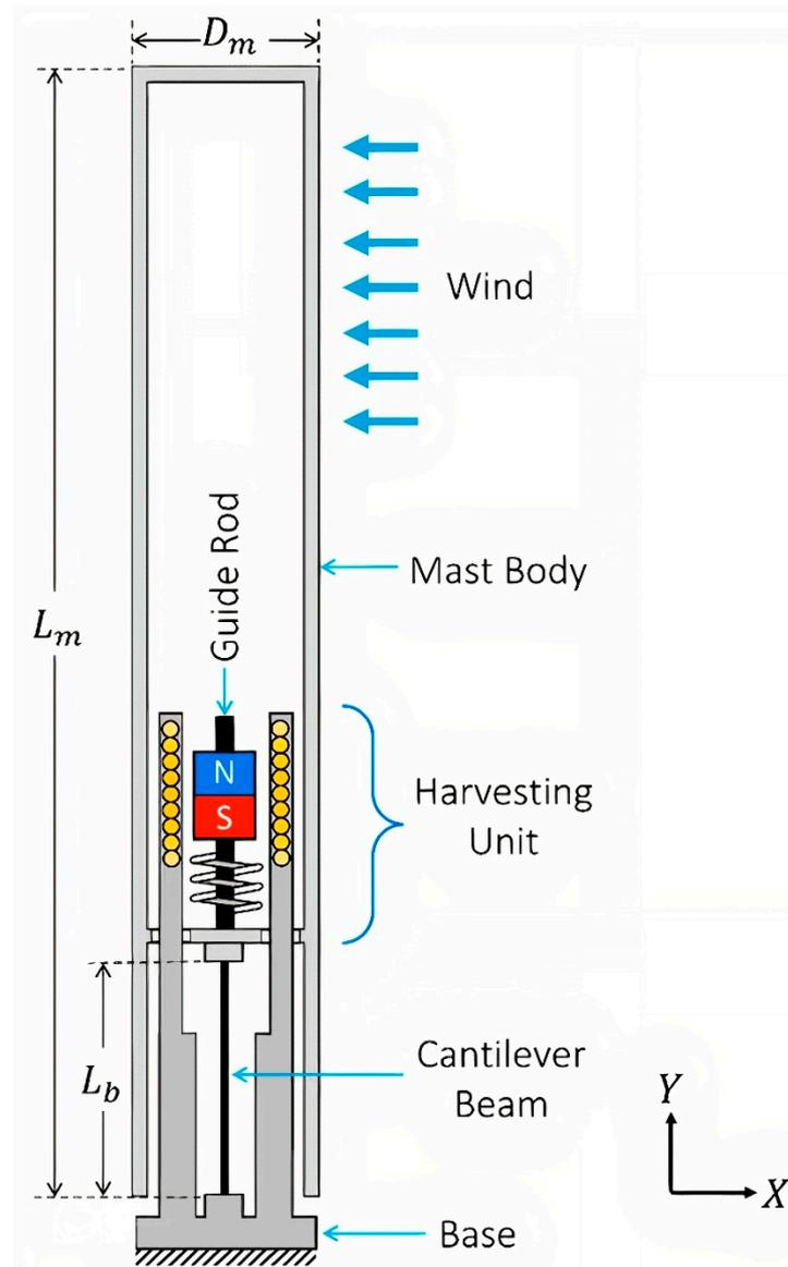
**Figure 4.** Schematic drawing of a bladeless wind turbine [69]. (Open Access).
