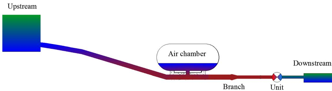
**Figure 1.** The pipeline system of the hydropower station with an ACSC.
