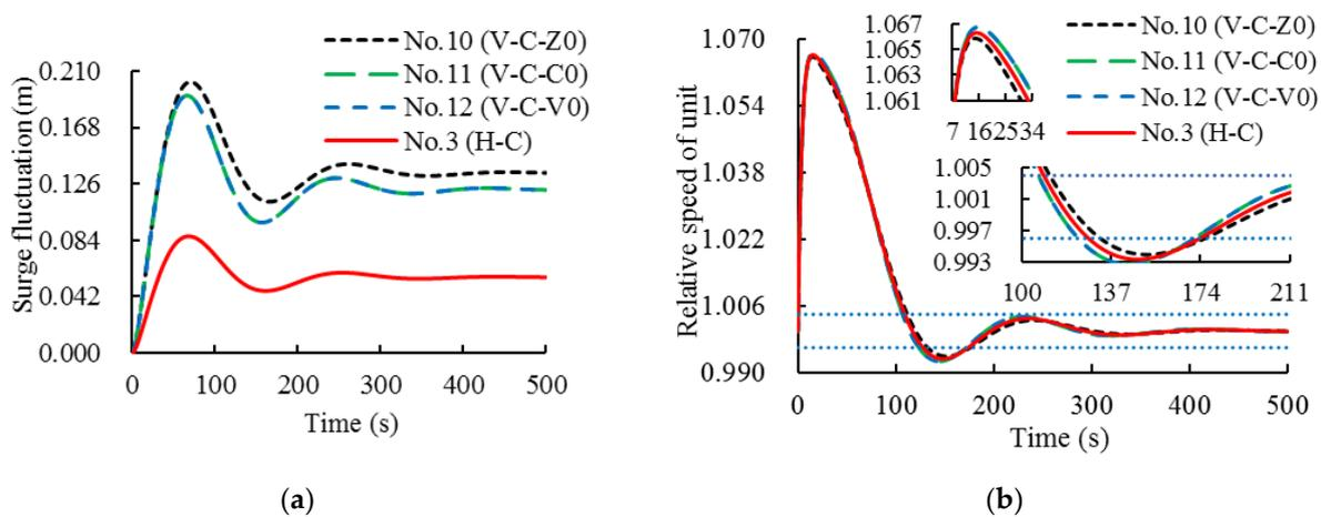
**Figure 5.** Comparison of horizontal and vertical ACSCs under SLD Condition C: (a) Surge varying with time; (b) Relative unit speed varying with time.
