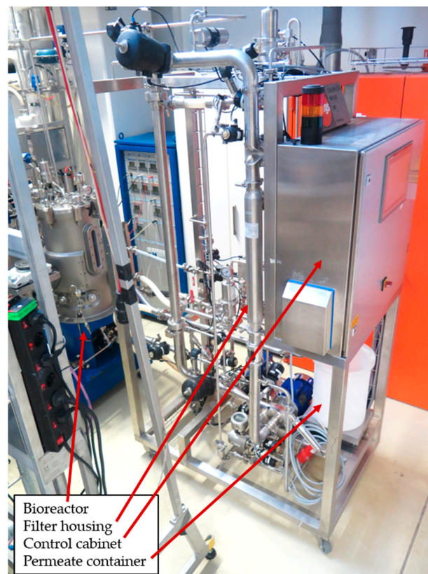
Figure 1. (a) Schematic illustration of the MBR system consisting of the stirred-tank bioreactor with a working volume of 50 L, a cross-flow microfiltration unit connected to it as an external bypass with a volume of 7.25 L, a 200 L feed tank, a permeate container, and peristaltic pumps for inlet and outlet streams; (b) a photograph of the steam-sterilizable MBR; (c) a photograph of the steam-sterilizable feed tank.
