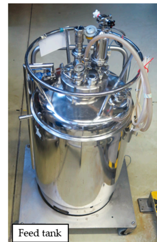
Figure 1. (a) Schematic illustration of the MBR system consisting of the stirred-tank bioreactor with a working volume of 50 L, a cross-flow microfiltration unit connected to it as an external bypass with a volume of 7.25 L, a 200 L feed tank, a permeate container, and peristaltic pumps for inlet and outlet streams; (b) a photograph of the steam-sterilizable MBR; (c) a photograph of the steam-sterilizable feed tank.
