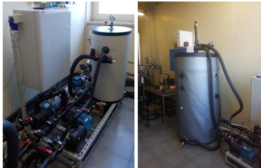
Figure 3. Picture of the testing rig installed at ITAE lab ( left-hand side ) and hybrid TES system connected under test conditions ( right-hand side ).
