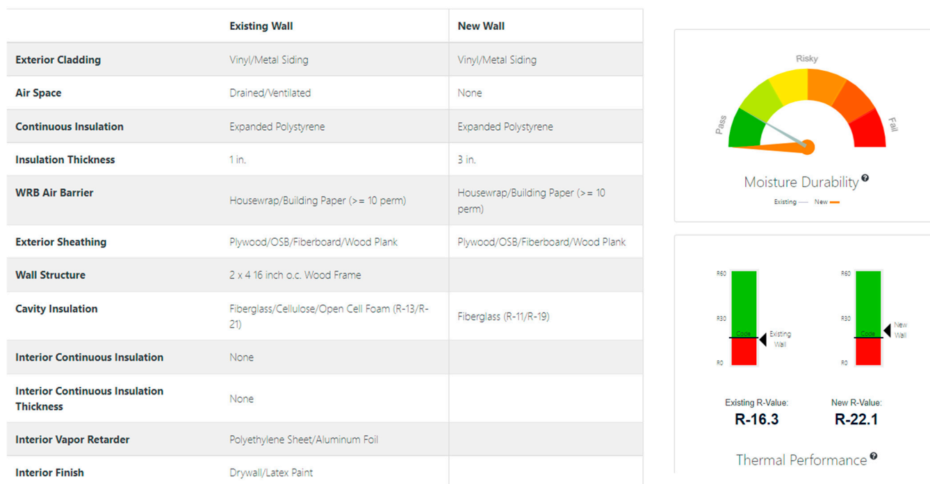
Figure 3. The final screen of the BSA retrofit tool comparing the materials and performance of the existing and proposed retrofit wall.
