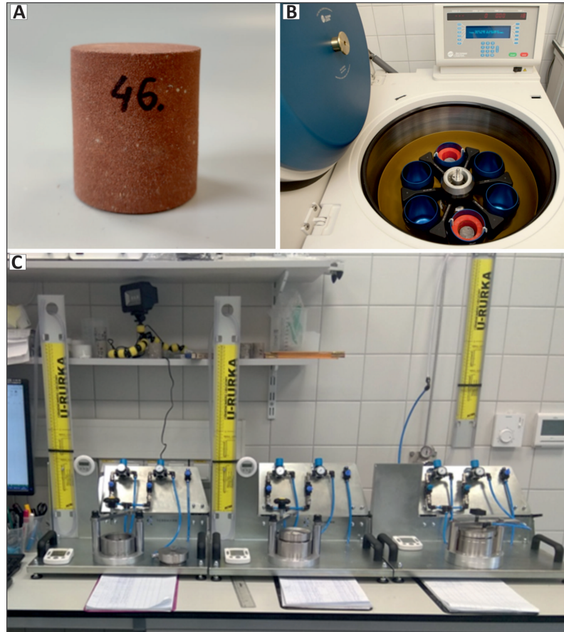
Figure 6. Core prepared for parameter determination (A), samples placed in a high-speed centrifuge (B), test equipment for measurement of k (C).
