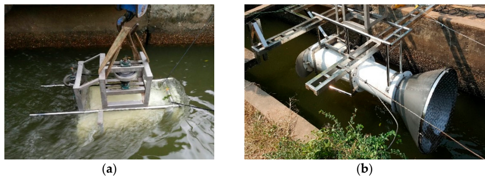
Figure 8. Field experiments. (a) The generator system with a diffuser as a trumpet-shaped collective chamber. (b) The generator system with an in-line pipe + diffuser + nozzle chamber.
