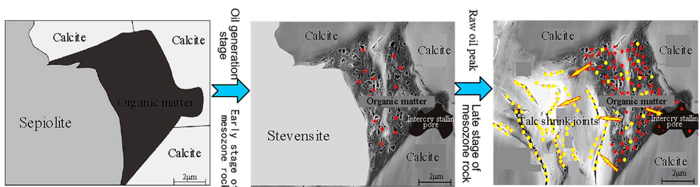
Figure 8. Diagram of the formation of organic pores and shrinkage joints in the talc transformation process.
