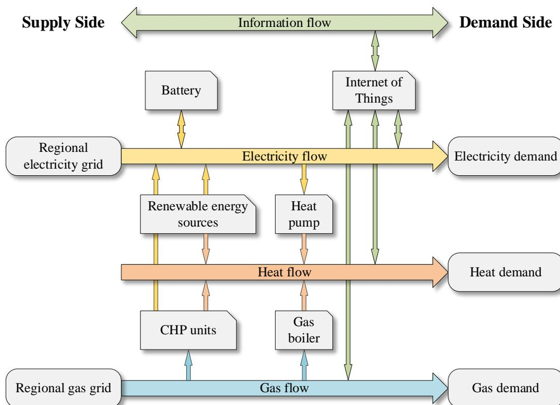
**Figure 1.** Schematic diagram of MES.
