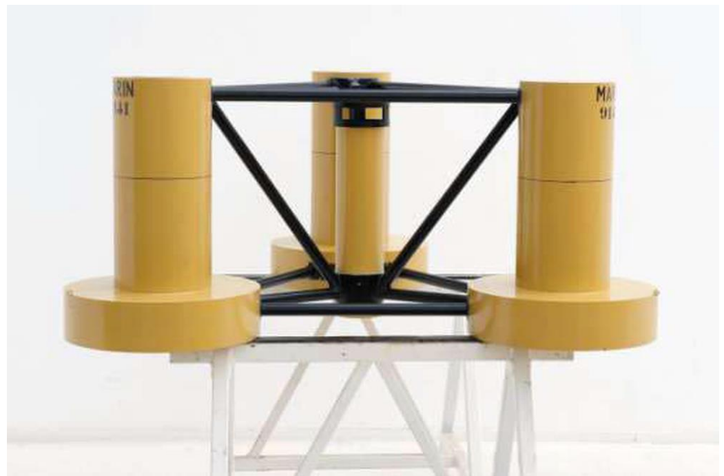
Figure 5. DeepCwind floating wind system design.
