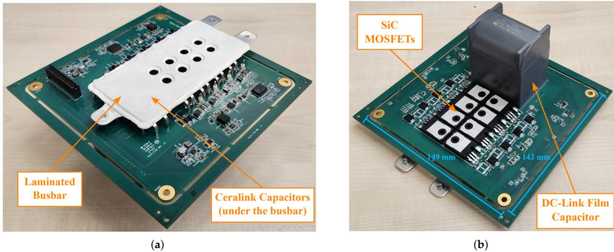
Figure 8. PCB images, (a) top side of the PCB, (b) bottom side of the PCB.
