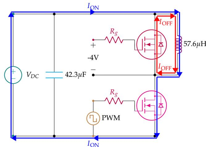
**Figure 2.** Double–pulse test (DPT) circuit.
