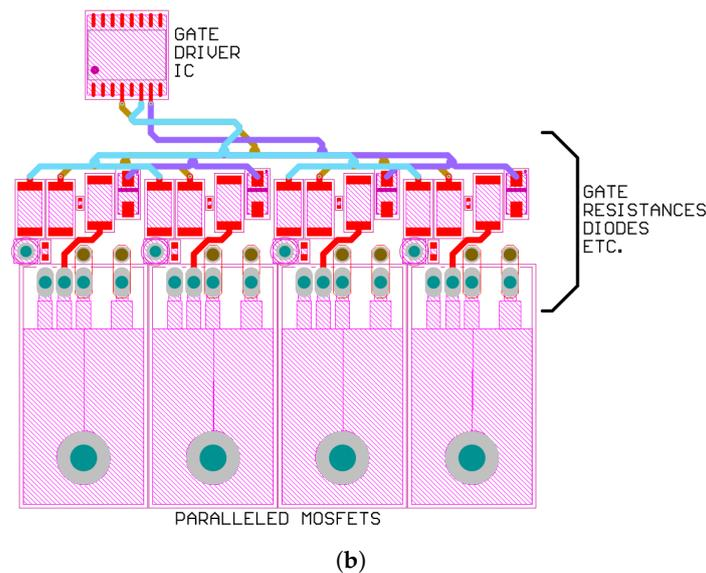
**Figure 4.** Layout of the gate driver circuit, (a) Gate turn-on path “yellow trace”, (b) gate turn-off path “blue trace”.
