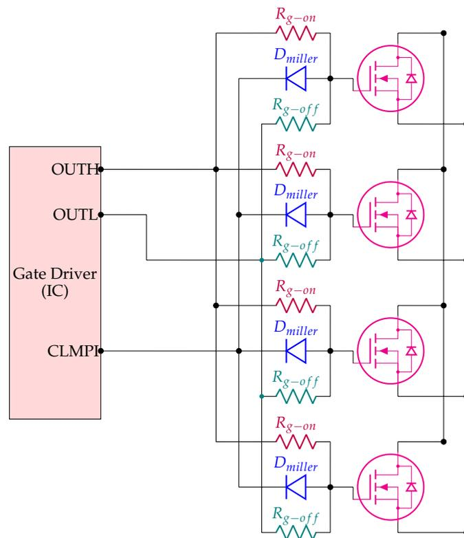
**Figure 5.** Schematic of Active Miller Clamp protection.
