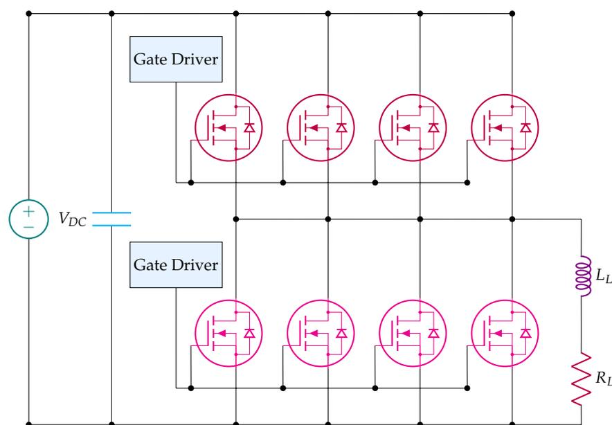
**Figure 1.** Proposed half-bridge topology with four paralleled SiC MOSFETs.
