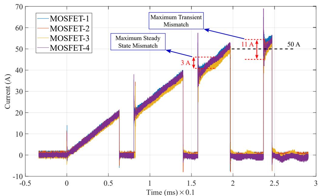
**Figure 15.** Paralleled SiC MOSFET currents.**Table 7.** Switching loss comparison.
