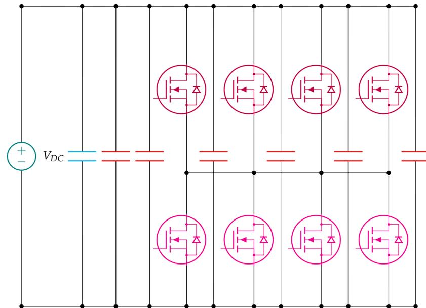
**Figure 10.** Location of 6  $\mu\text{F}$  Ceralink capacitance connected in parallel through discrete MOSFETs.
