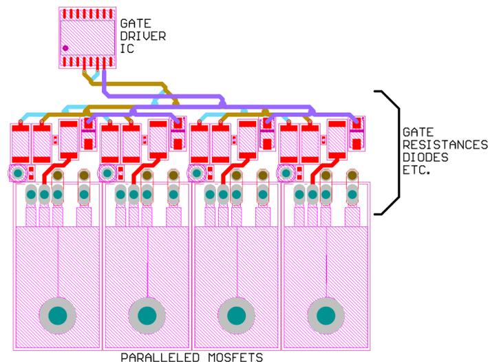
**Figure 6.** Layout of the Active Miller Clamp protection.
