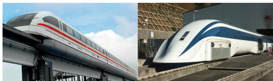
Figure 2. German TR08 Maglev train (left); Japanese MLX01 Maglev train (right).
