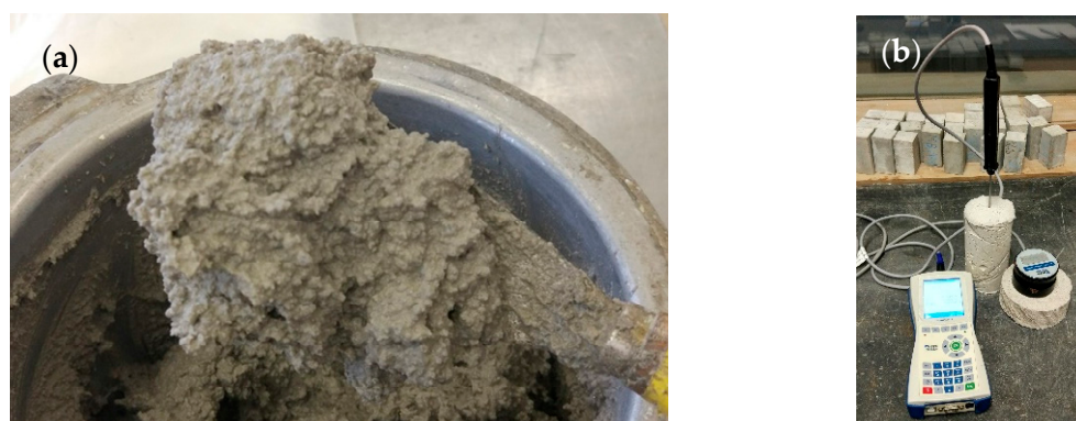
Figure 1. Aerogel-based render's visual aspect during the mixing process (a) and the specimens (cylindric I with a linear probe; closer—cylindric II with a plane probe) and ISOMET 2114 equipment from Applied Precision supplier (b).
