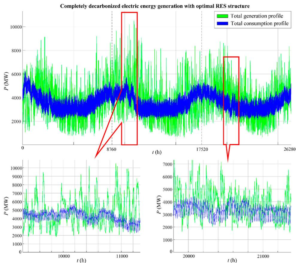
**Figure 9.** Total generation profile in completely decarbonized Serbian power system with optimized RES capacities.
