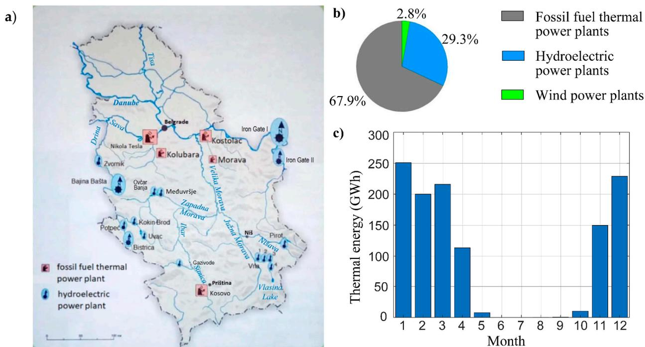
**Figure 2.** (a) Electric power plants in Serbia; (b) electrical energy generation structure in Serbia; (c) thermal energy produced in cogeneration power plants in Serbia.
