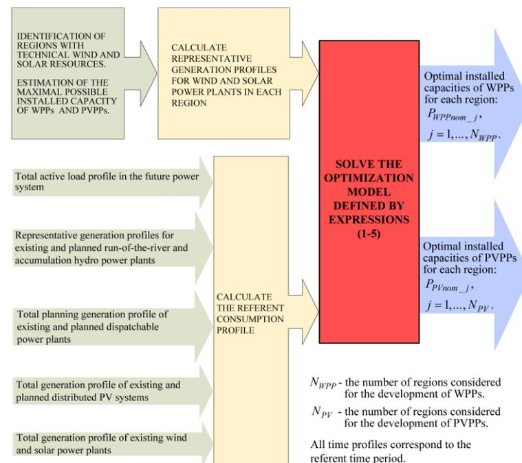
**Figure 1.** The proposed algorithm for planning RES development for complete decarbonization of electrical energy generation.
