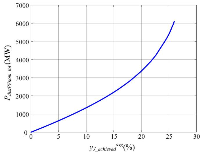
**Figure 5.** The required installed capacity of distributed PV systems for achieving a certain weighted average value of Joule’s losses reductions in distribution networks in Serbia.
