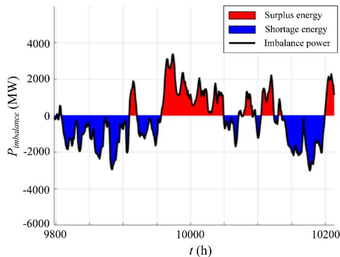
**Figure 10.** The imbalance power profile with surplus and shortage energy.
