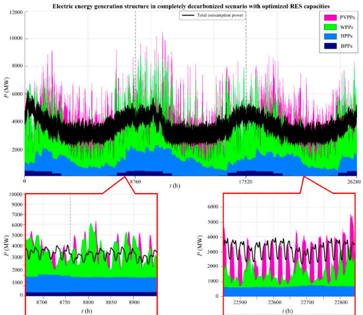
Figure 8. Different generation technology shares in the total generation profile.
