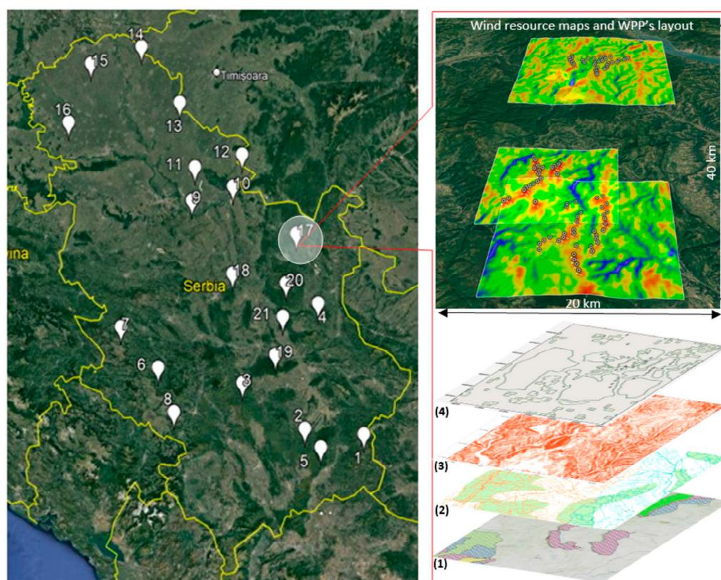
**Figure 3.** Positions of the measuring points in the identified windy regions in Serbia (denoted by numbers 1–21) with the illustration of the wind energy potential estimation for a single target region. Layers: (1) Nature protected areas, (2) Urbanism and infrastructure, (3) Orography, (4) Roughness.
