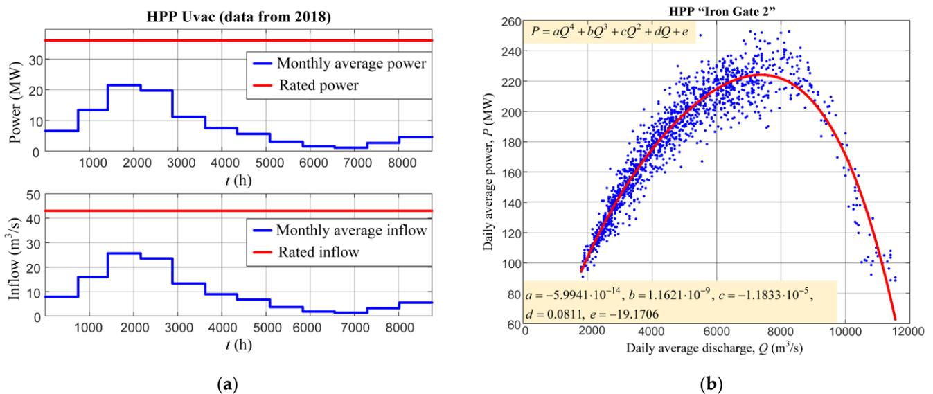
**Figure 6.** (a) Representative generation profile for HPP “Uvac”; (b) representative generation curve for HPP “Iron Gate 2”.
