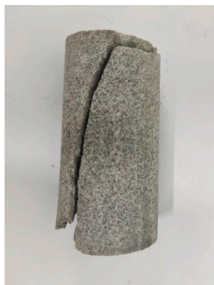
Figure 3. Triaxial compression test phenomenon of the sand hydrate sample.
