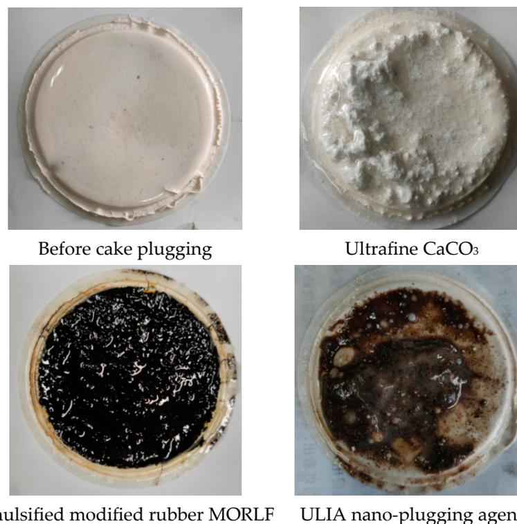
**Figure 4.** Comparison chart of filter cake before and after plugging.
