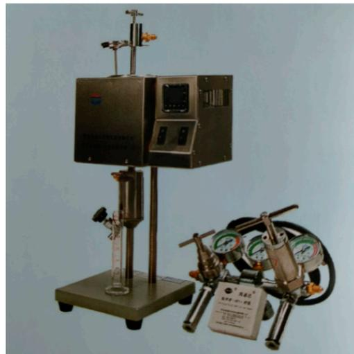
**Figure 1.** High temperature and pressure filtration instrument.
