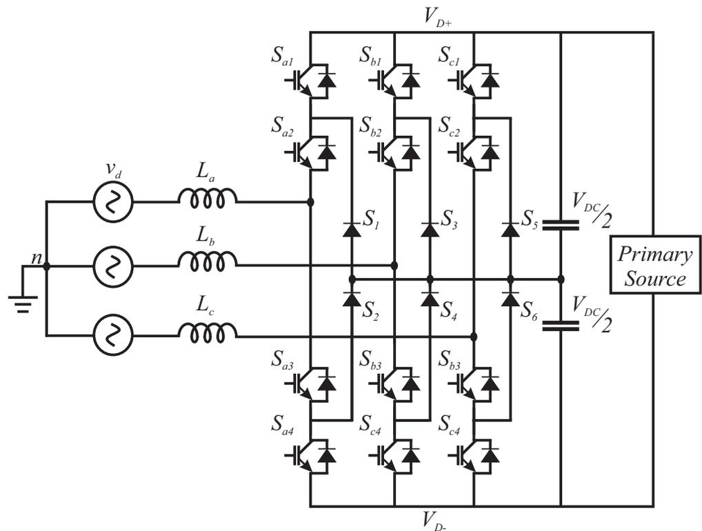
**Figure 5.** Three-Level NPC Converter Topology.
