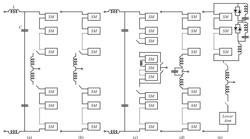
**Figure 8.** Parallel-Connected Topologies: (a) Short Overlap, (b) Extended Overlap, (c) Shared Alternate Arm, (d) Improved Alternate Arm, (e) Augmented Trapezoidal Arm.
