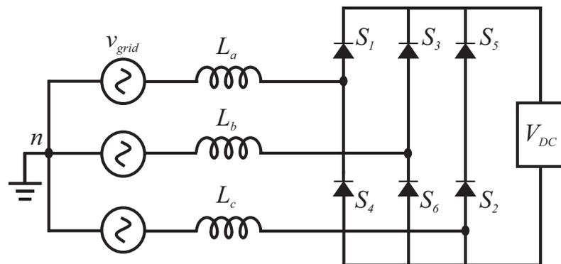
**Figure 2.** Six-Pulse Converter Topology.
