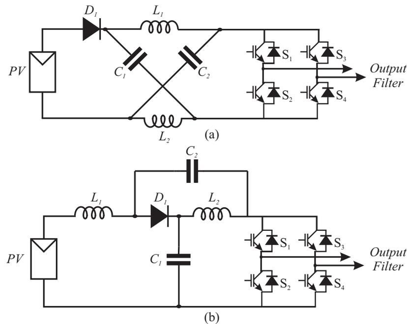
**Figure 10.** Z-source and quasi-Z-source converter topologies. (a) ZSI; (b) qZSI.
