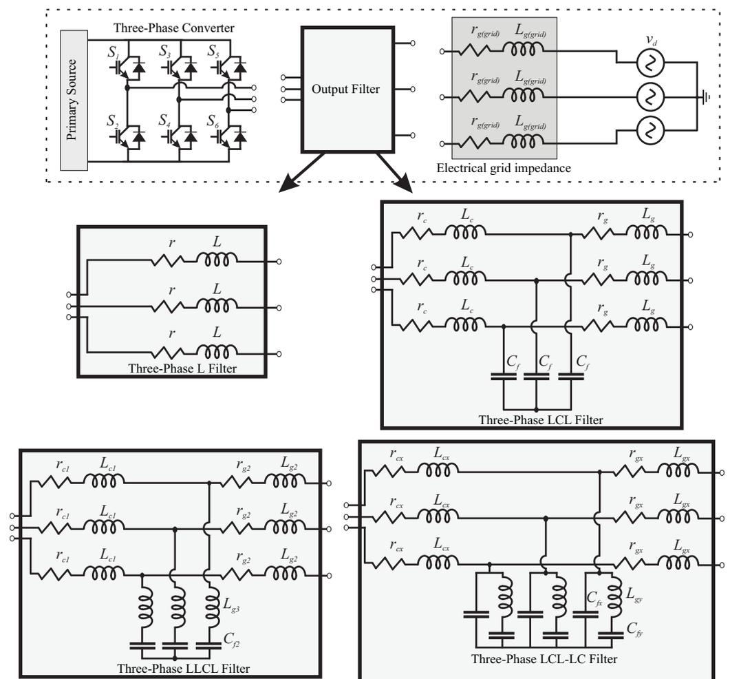
**Figure 11.** General three-phase grid-connected power converter diagram with L, LCL, LLCL, and LCL-LC filters.
