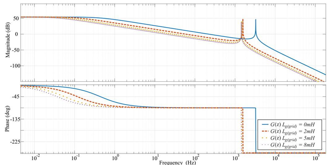
**Figure 13.** Bode diagram of a grid-connected converter with LCL filter under grid impedance variation.
