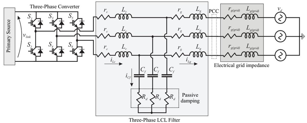
**Figure 12.** Diagram of a general three-phase grid-connected converter with an LCL filter.
