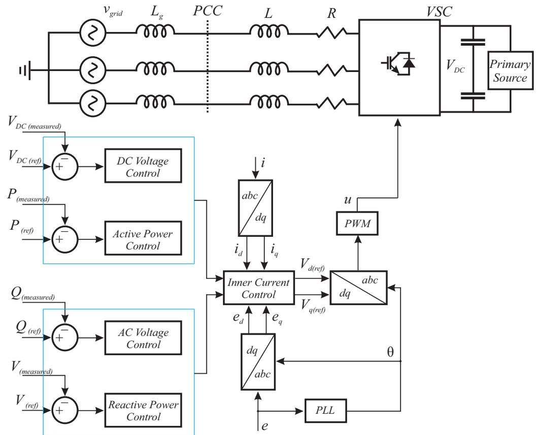
Figure 6. Vector-Controlled VSC Architecture.
