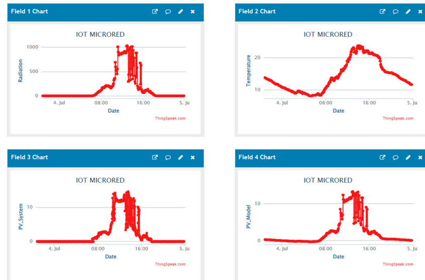
Figure 6. Results of PV monitoring in real-time online.
