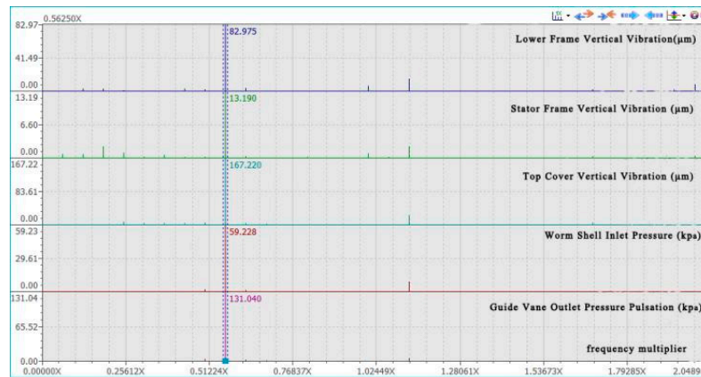
Figure 8. Harmonic ratio graph of vibration measurement pressure during unit operation at 80.449% openness.
