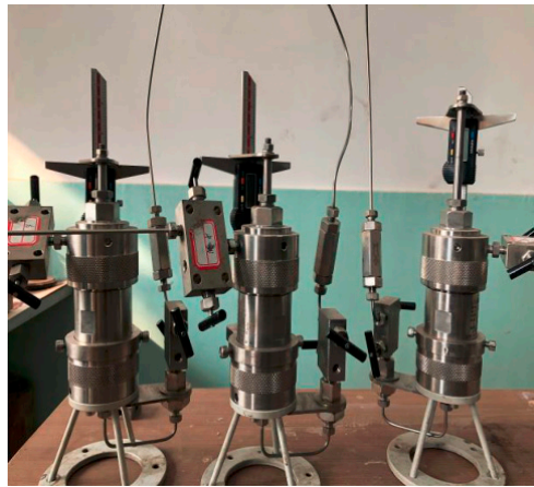
Figure 3. High-temperature–high-pressure extremely low-flow dynamic monitoring system.
