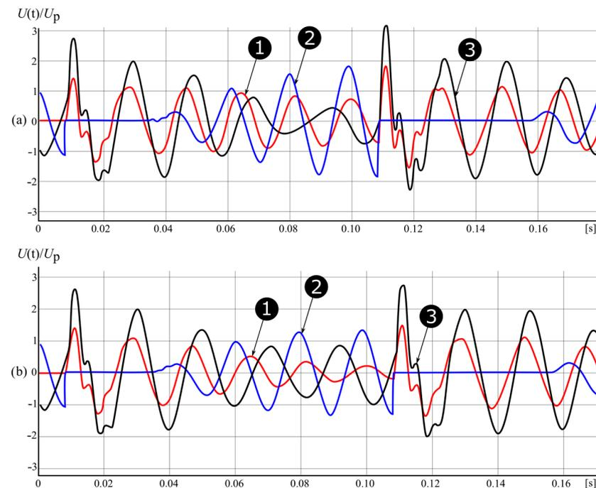
**Figure 10.** Waveforms of voltages in the event of a re-occurrence of a short-circuit after its short-circuit extinction in a compensated MV network with significant detuning ( $s = 0.2$ ) for two cases: for  $d_0 = 0.04$  (graph a) and for  $d_{0W} = 0.14$  (graph b) (1—neutral point voltage, 2—earth phase voltage, 3—healthy phase voltage).
