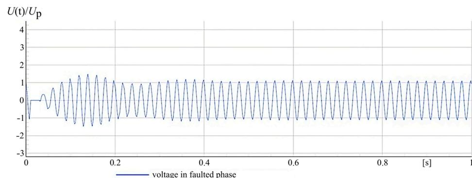
**Figure 3.** Waveform of the phase voltage of the faulted MV network after the disappearance of the earth fault in the overcompensated network ( $s = 0.2$ ) with natural damping coefficient  $d_0 = 0.04$ .
