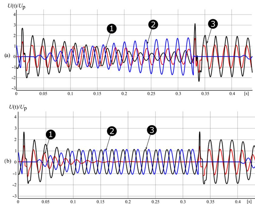
**Figure 9.** Waveforms of voltages in the event of a re-occurrence of a short-circuit after its short-circuit extinction in the compensated MV network ( $s = 0$ ) for two cases: for  $d_0 = 0.04$  (graph a) and for  $d_{0W} = 0.14$  (graph b) (1—neutral point voltage, 2—earth phase voltage, 3—healthy phase voltage).
