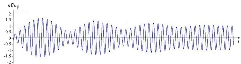
**Figure 6.** The process of restoring the voltage of the earthed phase after the disturbance disappearance, recorded in a network with high compensation detuning ( $s = 0.3$ ,  $d_0 = 0.04$ ).
