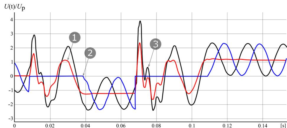
**Figure 8.** Waveforms of voltages in the event of a re-occurrence of a short-circuit after its short-circuit extinction in the MV network with an insulated neutral point. (1—neutral point voltage, 2—earth phase voltage, 3—healthy phase voltage).
