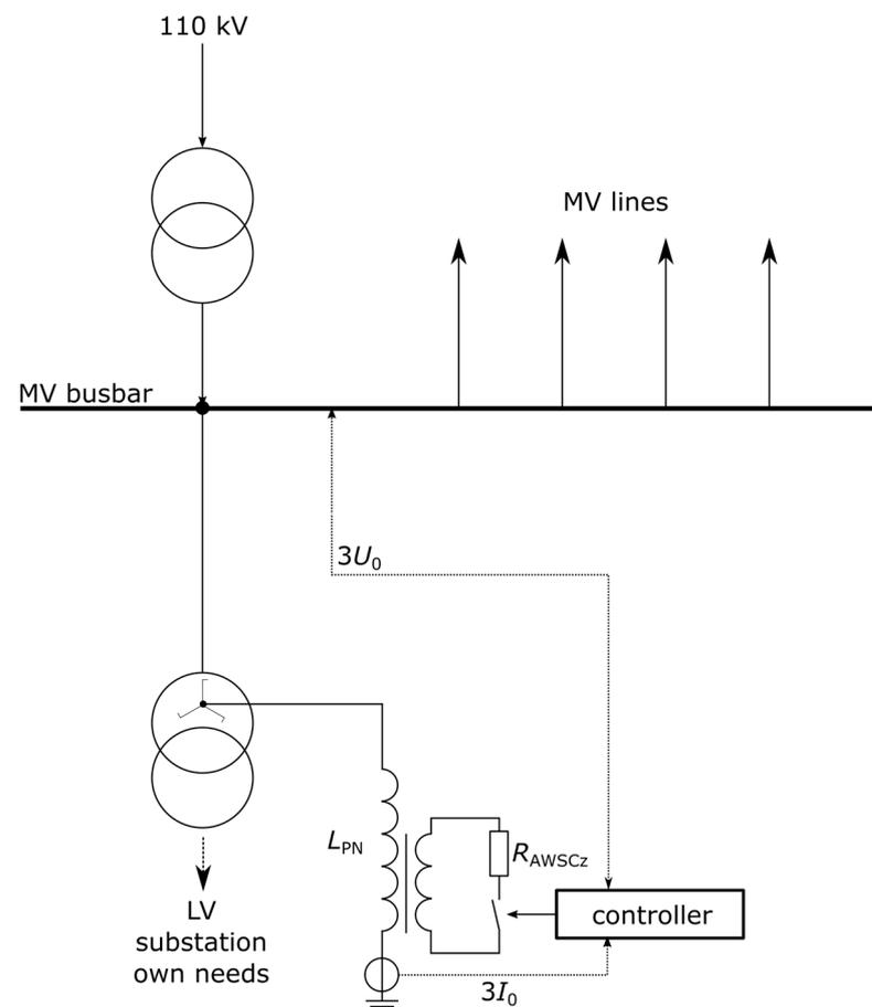
**Figure 1.** AWSCz forcing system with forcing resistor connected to the additional one low-voltage winding of the compensating coil  $L_{PN}$ .
