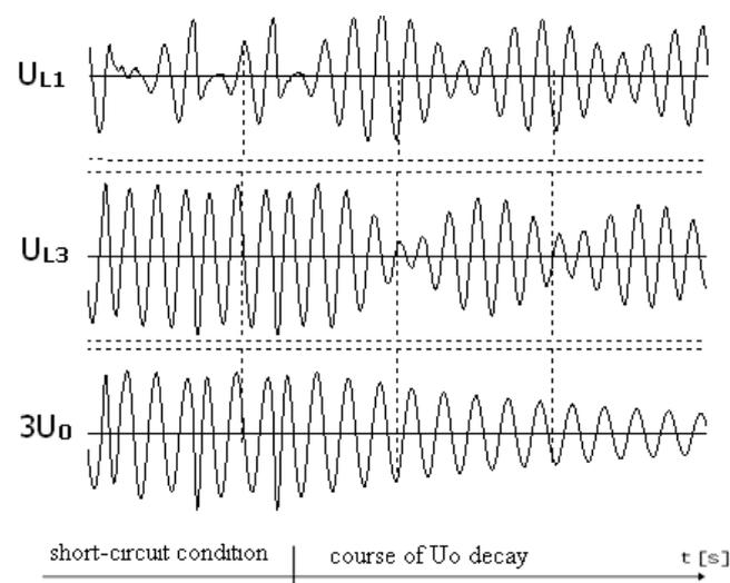
**Figure 7.** Voltage waveforms in a real 15 kV network recorded during an intermittent arc earth fault in the L1 phase [22].
