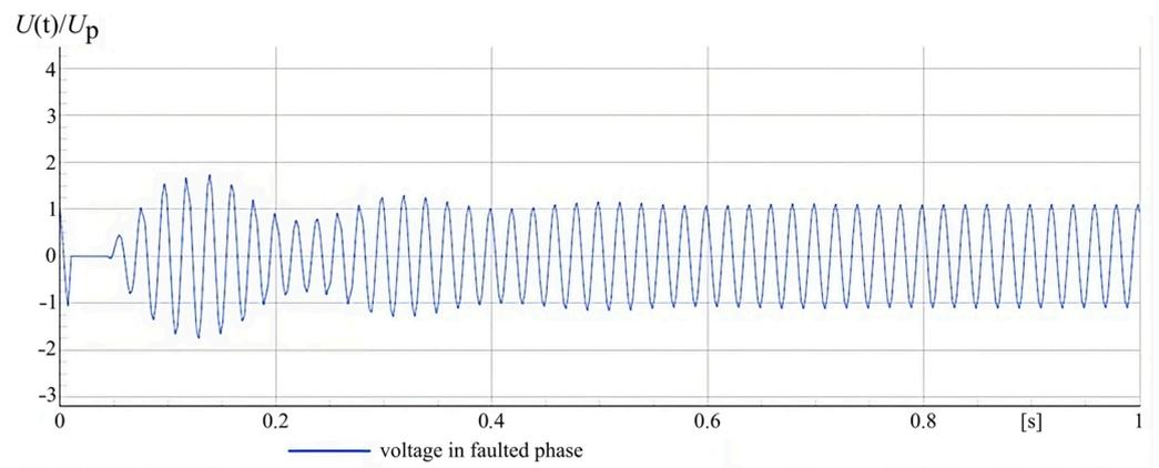
**Figure 4.** Waveform of the phase voltage of the faulted MV network after the disappearance of the earth fault in the uncompensated network ( $s = -0.2$ ) with natural damping coefficient  $d_0 = 0.04$ .
