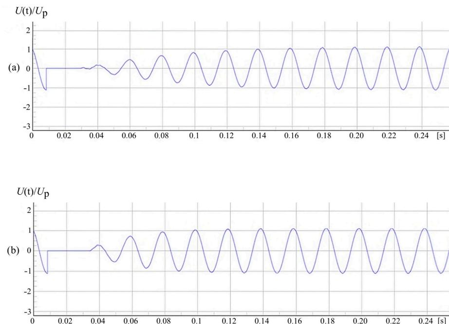
**Figure 5.** Voltage waveform of the faulted phase after the short-circuit disappearance in the compensated network ( $s = 0.05$ ) and damping coefficients  $d_{0W} = 0.1$  (graph (a)) and  $d_{0W} = 0.25$  (graph (b)).
