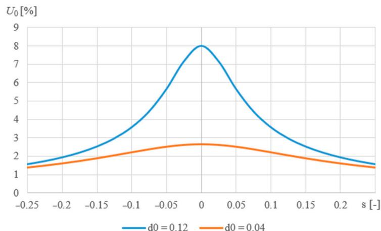
**Figure 2.** Curves of the zero-sequence voltage of the network  $U_0$  in a compensated network with earth asymmetry at the level of 0.45%, depending on the degree of compensation detuning and the value of the damping coefficient  $d_0$ .
