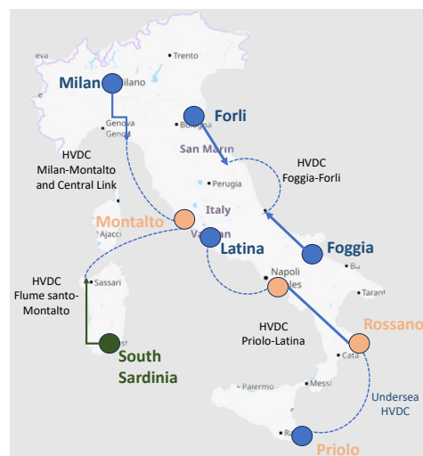
Figure 5. Hypergrid project in Italy [19].
