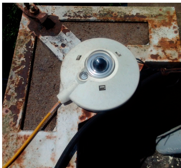
Figure 2. Pyranometer used to measure GHI during the campaign.
