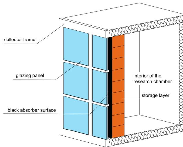
**Figure 6.** Construction of the thermal storage wall.
