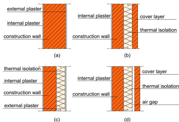
**Figure 2.** Traditional solutions for the construction of external masonry walls: (a) one-layer wall (L1); (b) three-layer wall (L3); (c) two-layer wall (L2); (d) three-layer wall with hollow core (L3).
