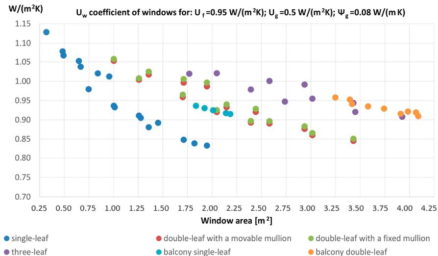
**Figure 4.**  $U_w$  coefficient of windows of various designs for a classic spacer frame with coefficient  $\Psi_g = 0.08$ .
