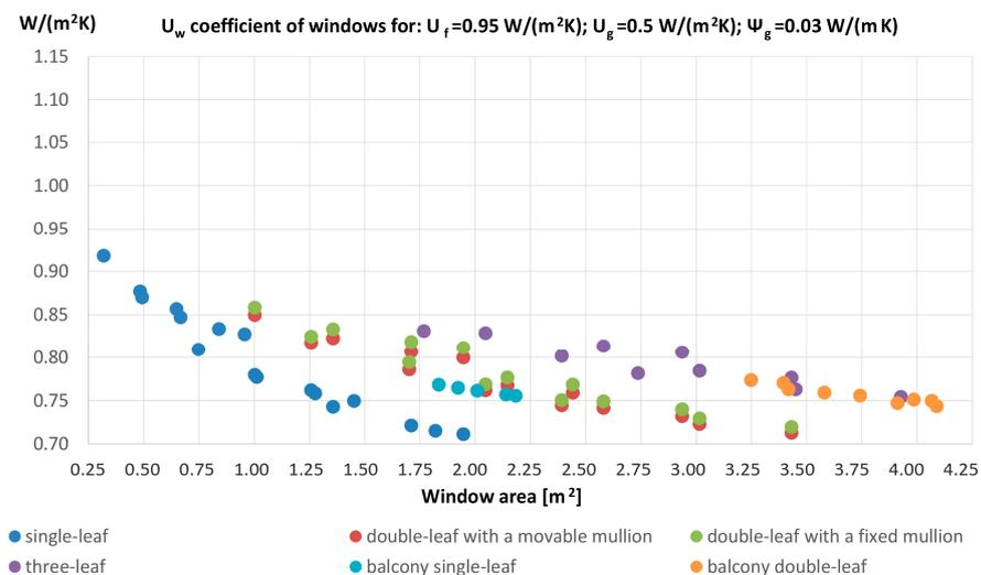
**Figure 5.**  $U_w$  coefficient of windows of various designs for a “warm” spacer with coefficient  $\Psi_g = 0.03$ .
