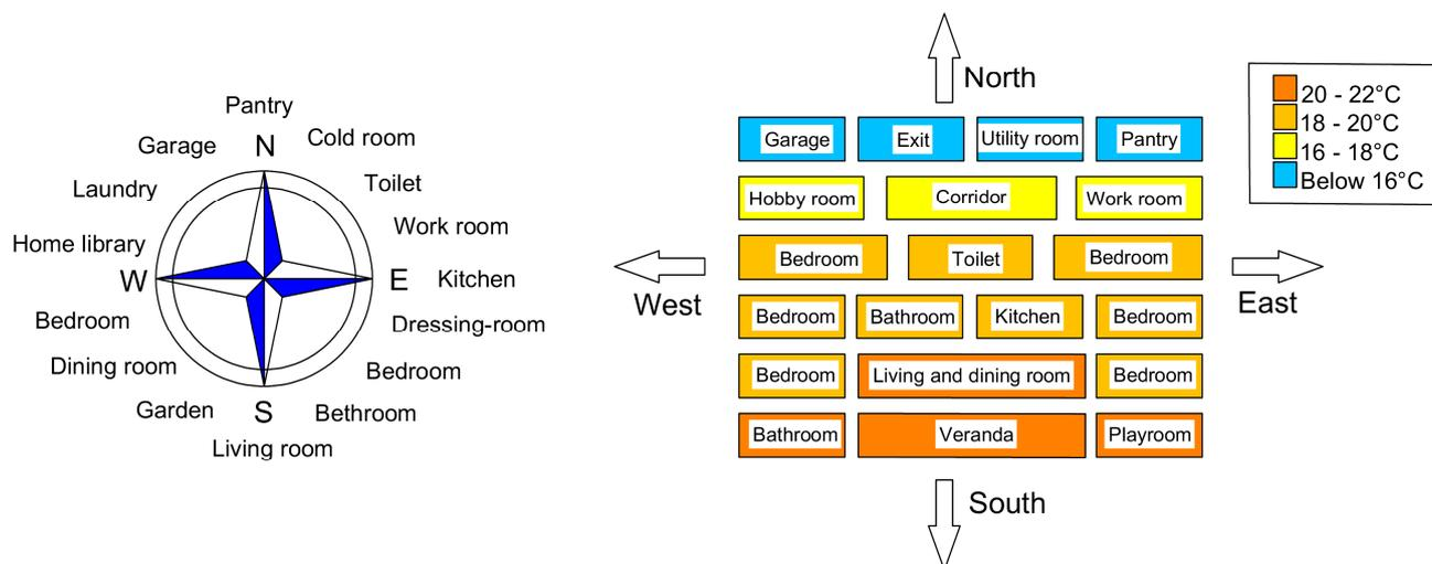
**Figure 1.** Sample arrangement of rooms relative to cardinal directions.
