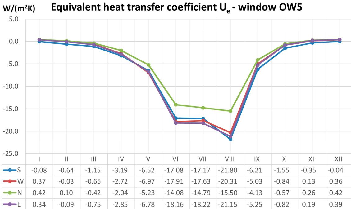
**Figure 7.** Equivalent heat transfer coefficient  $U_e$  of the OW5 window for four orientations.
