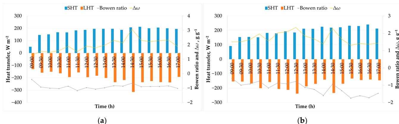
**Figure 6.** Variation in the sensible and latent heat transfer as a function of time: (a) luffa pad; (b) luffa pad + external shading net.
