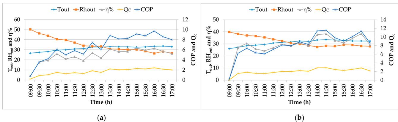
**Figure 7.** Variations of performance parameters the SNP and SNP + ESN pads with time (a) SNP; (b) SNP + ESN.
