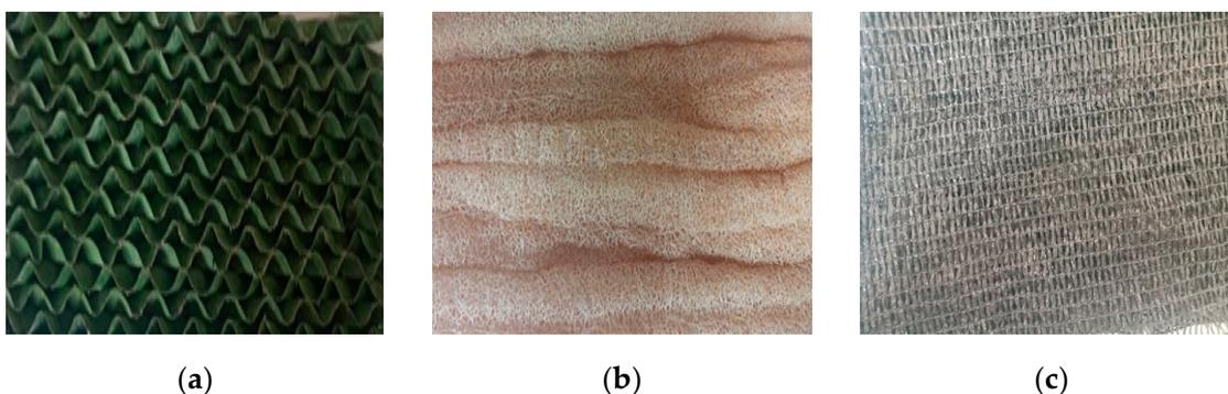
**Figure 2.** The testing materials: (a) cellulose pad; (b) luffa pad; (c) shading net pad.
