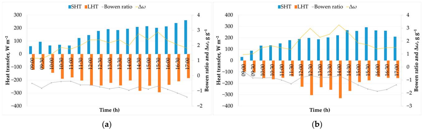
**Figure 4.** Variation in the sensible and latent heat transfer as a function of time: (a) cellulose pad; (b) cellulose pad + external shading net.
