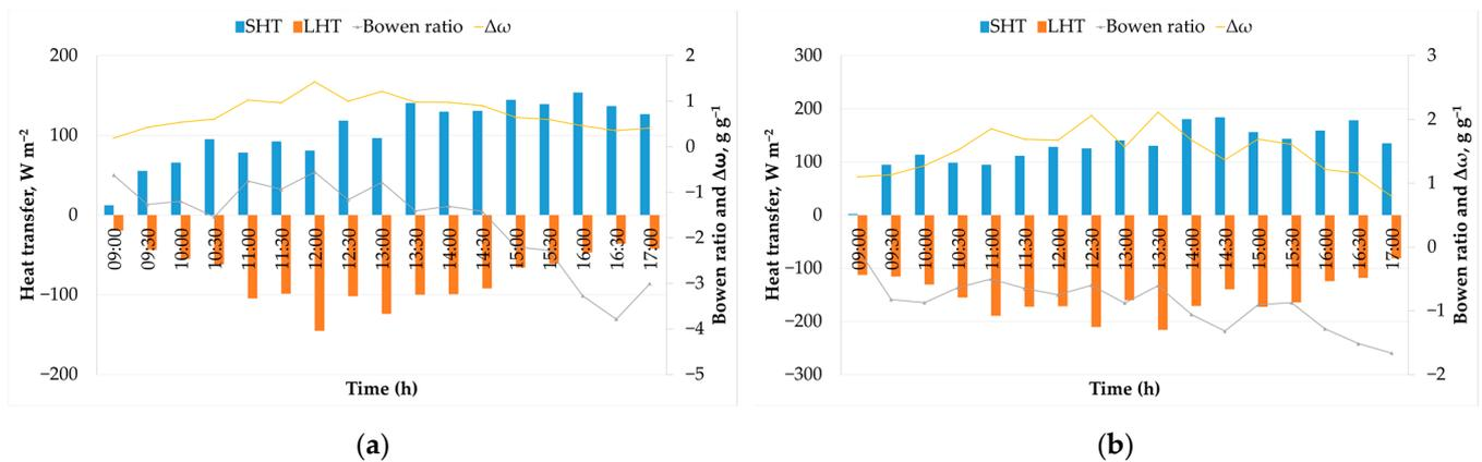
**Figure 8.** Variation in the sensible and latent heat transfer as a function of time: (a) shading net pad; (b) shading net pad + external shading net.
