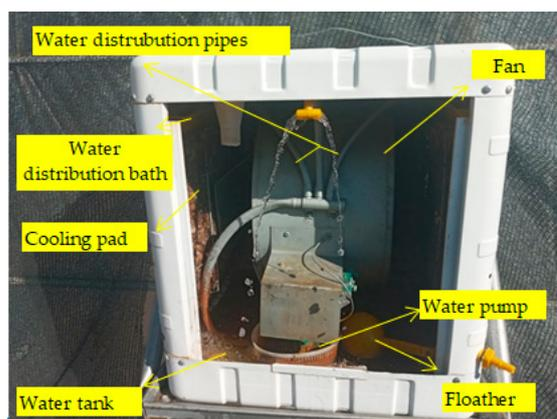
**Figure 1.** Direct evaporative cooling system and the components of the system.
