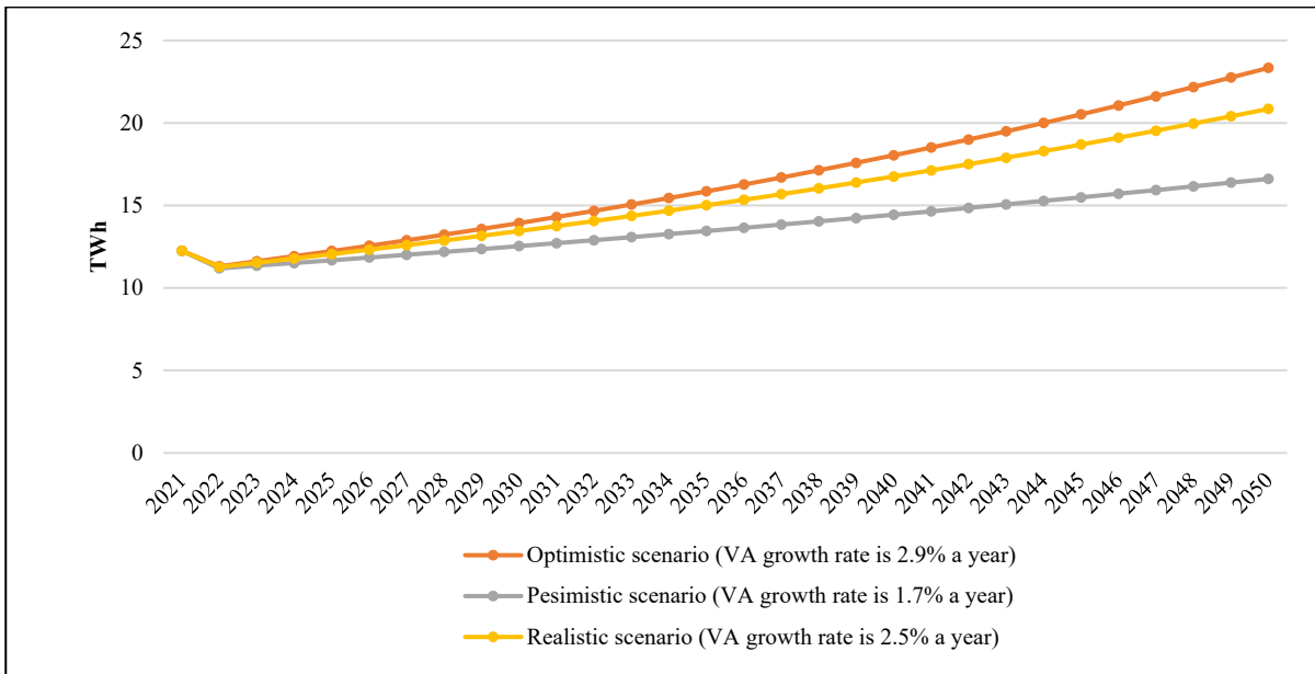
Figure 16. Forecasts of final energy consumption in the Lithuanian manufacturing industry from 2022 to 2050 subject to different value-added growth scenarios, TWh (own estimations).
