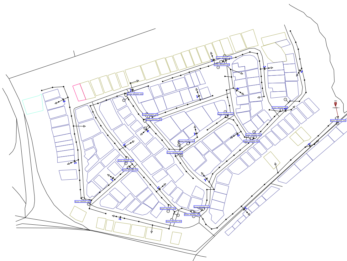
Figure 3. Georeferenced area created with QGIS, including system nodes in an actual urban distribution network.
