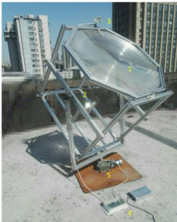
**Figure 29.** The concentrating reactor system. 1. Concentrating mirror; 2. Reactor; 3. Sensor for tracing sun; 4. Controller; 5. Motor. Reproduced by kind permission of Elsevier from [168].
