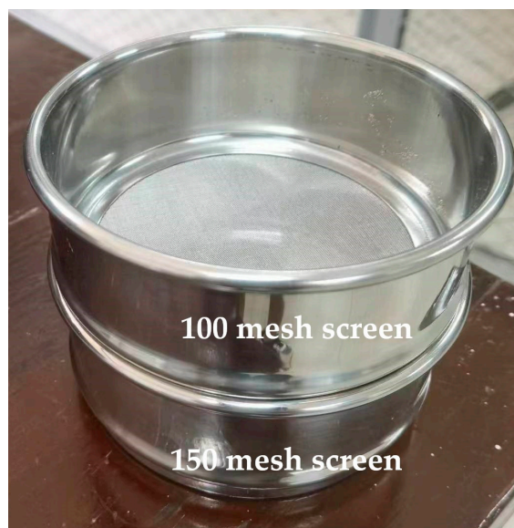
Figure 3. Illustration of 100-mesh and 150-mesh screens.
