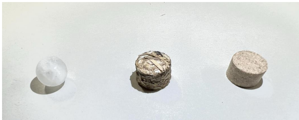
Figure 1. Example of feedstock samples (polypropylene, wheat straw, and poplar from left to right).
