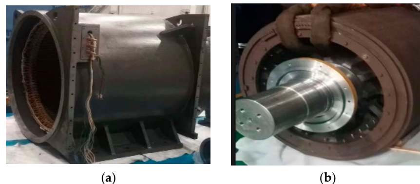
Figure 23. The surface-mounted rotor structure prototype: (a) stator and (b) rotor.
