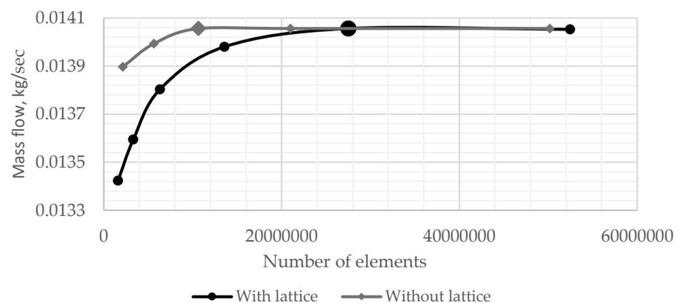
**Figure 12.** Mesh independence test results.
