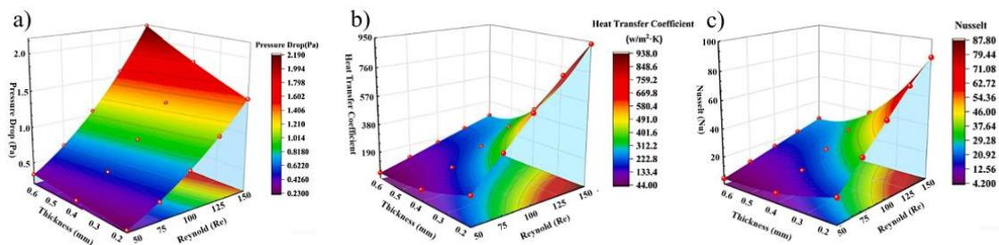
**Figure 8.** Plots of pressure drop (a), heat transfer coefficient (b) Nusselt number (c) dependence on gyroid lattice wall thickness and Reynolds number.
