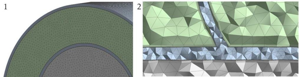
**Figure 13.** Mesh model: (1)—view from the flow inlet side; (2)—cross-sectional view.
