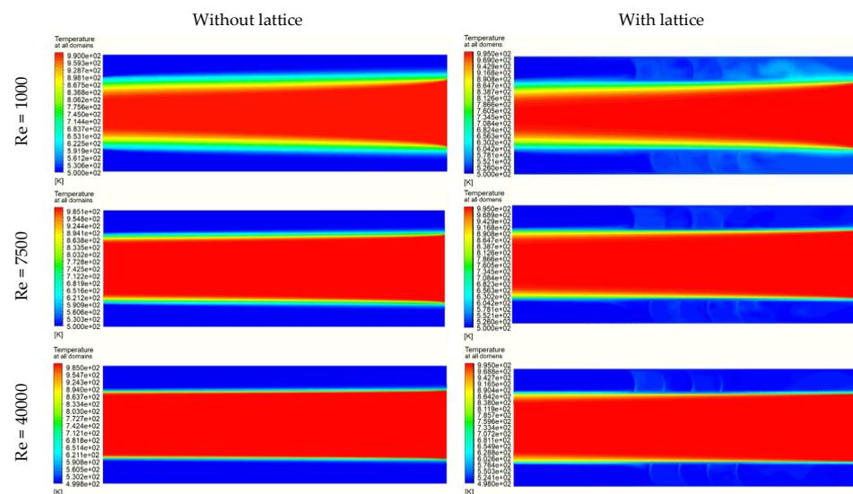
Figure 16. Temperature distribution in all domains of the heat exchanger for different calculation variants.
