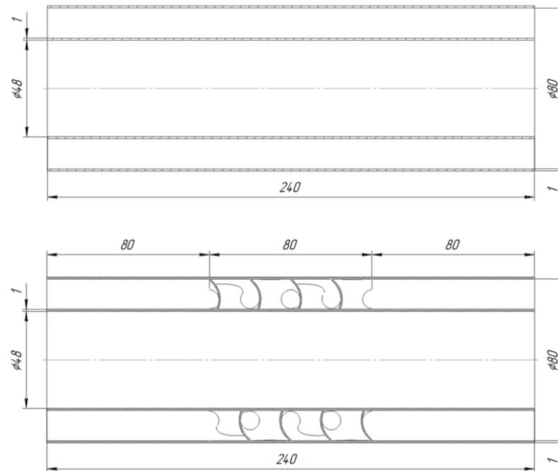
**Figure 10.** Sketch of heat exchanger sections.
