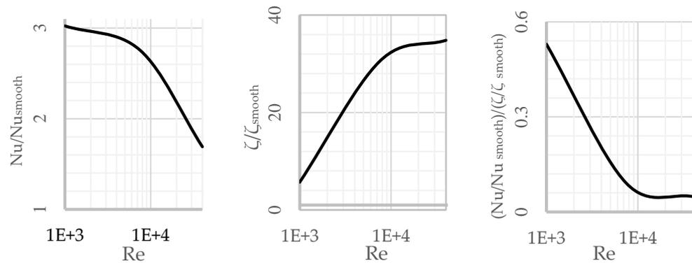
**Figure 21.** Plots of dependence of parameters  $Nu/Nu_{smooth}$ ,  $\zeta/\zeta_{smooth}$  and  $\frac{Nu/Nu_{smooth}}{\zeta/\zeta_{smooth}}$  of  $Re$  number for the investigated model of the heat exchanger section with gyroid lattice.
