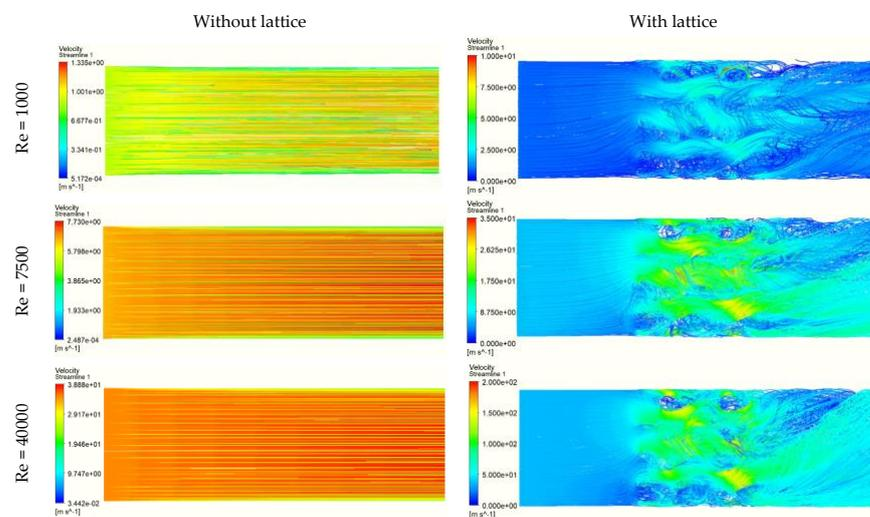
Figure 19. Current lines (velocities) in the cooler domain for different calculation variants.
