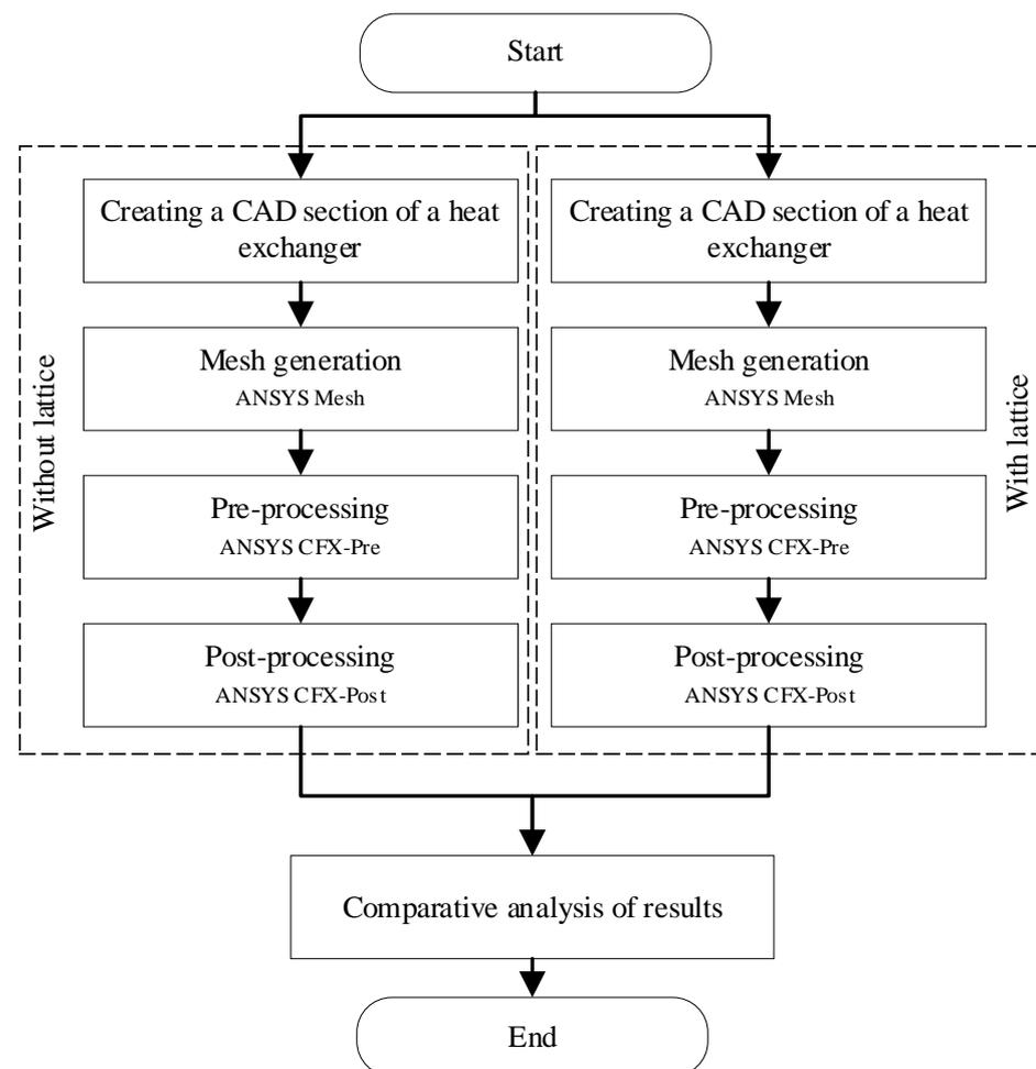
**Figure 9.** Block diagram of the study of heat transfer intensification through the use of gyroid lattice structures.
