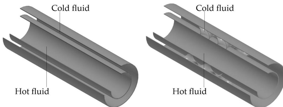
**Figure 11.** Geometric models of the studied heat exchanger sections in cross-section.
