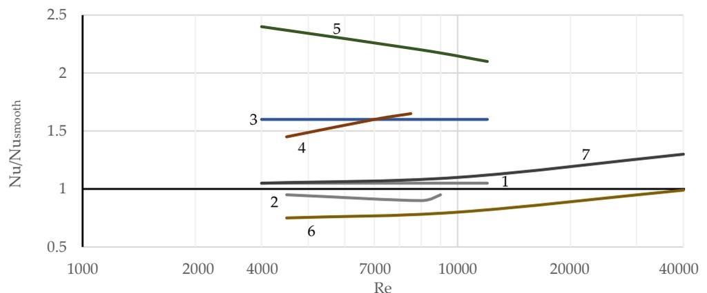
**Figure 3.** Dependence of  $Nu/Nu_{smooth}$  parameter on  $Re$  number for tube bundles with different types of finning: 1—longitudinal continuous finning; 2—longitudinal finning in close bundles; 3—longitudinal perforated finning; 4—longitudinal incised finning with rib rotation; 5—longitudinal incised finning with edge bending; 6—transverse continuous ribbing; 7—transverse petal ribbing.
