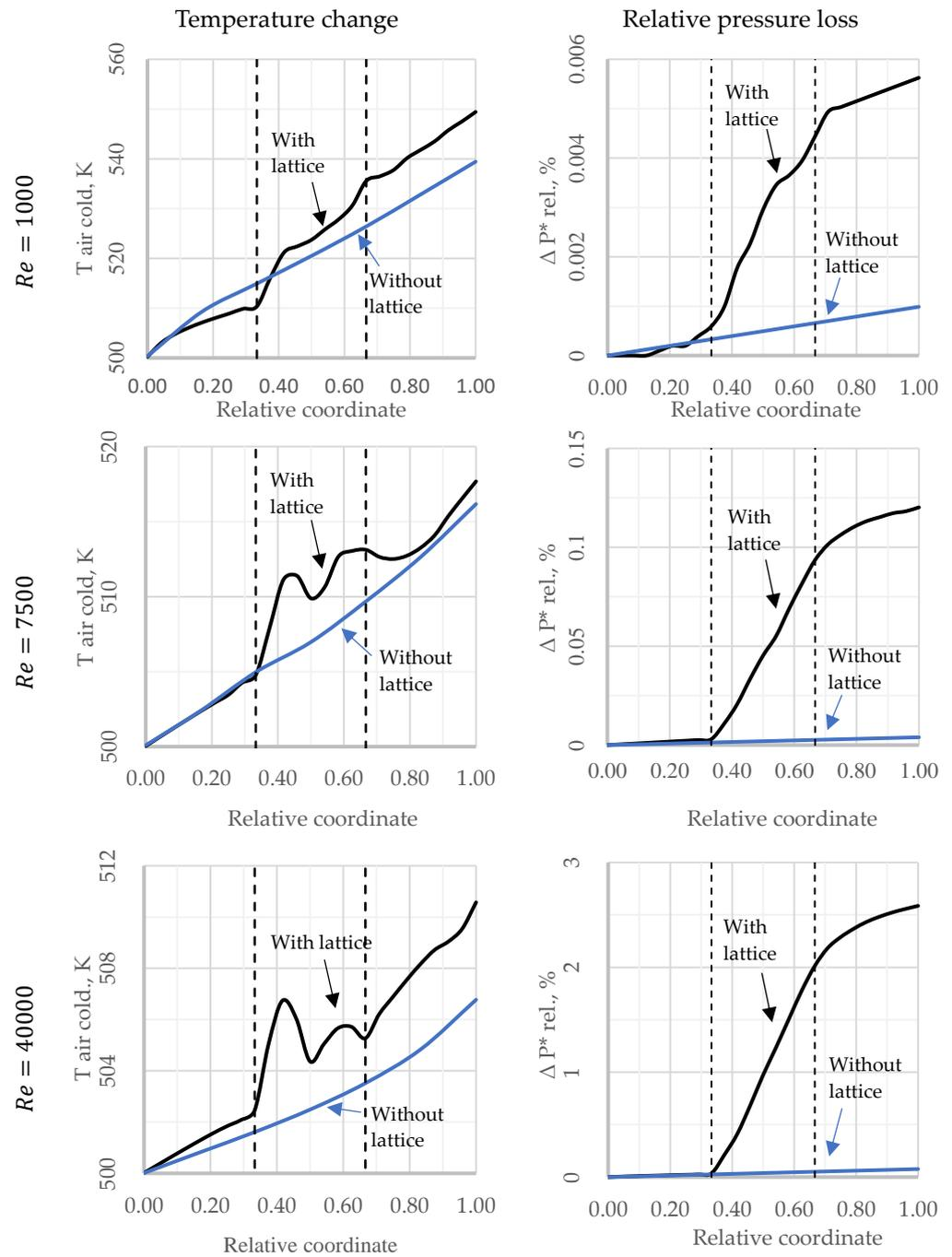
**Figure 20.** Plots of temperature change and value of relative losses of total pressure as the heat exchanger section passes through for heat exchanger sections with and without grids at different Reynolds numbers.
