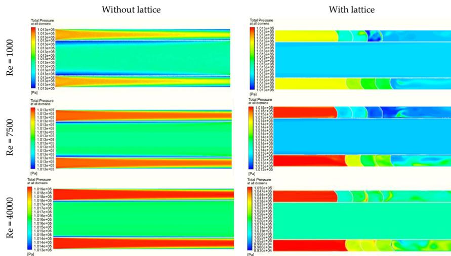
Figure 18. Full pressure distribution in all domains of the heat exchanger for different calculation variants.
