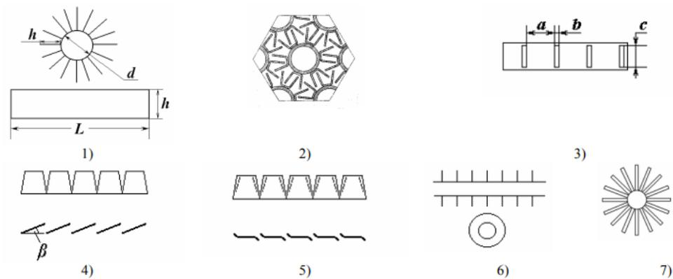
**Figure 2.** Surfaces with different types of finning: (1)—longitudinal continuous finning; (2)—longitudinal finning in close bundles; (3)—longitudinal perforated finning; (4)—longitudinal incised finning with rib rotation; (5)—longitudinal incised finning with edge bending; (6)—transverse continuous ribbing; (7)—transverse petal ribbing.
