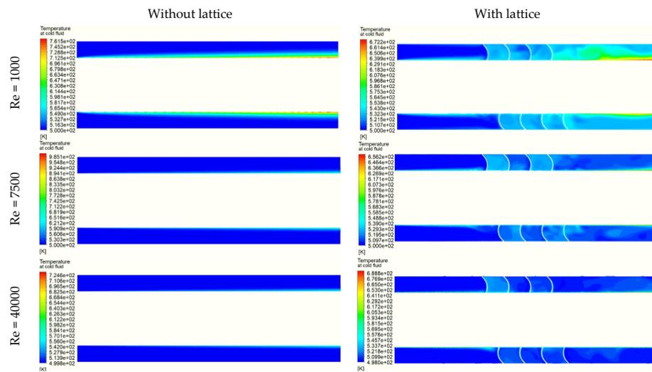
Figure 17. Temperature distribution in the cold domain for different calculation variants.
