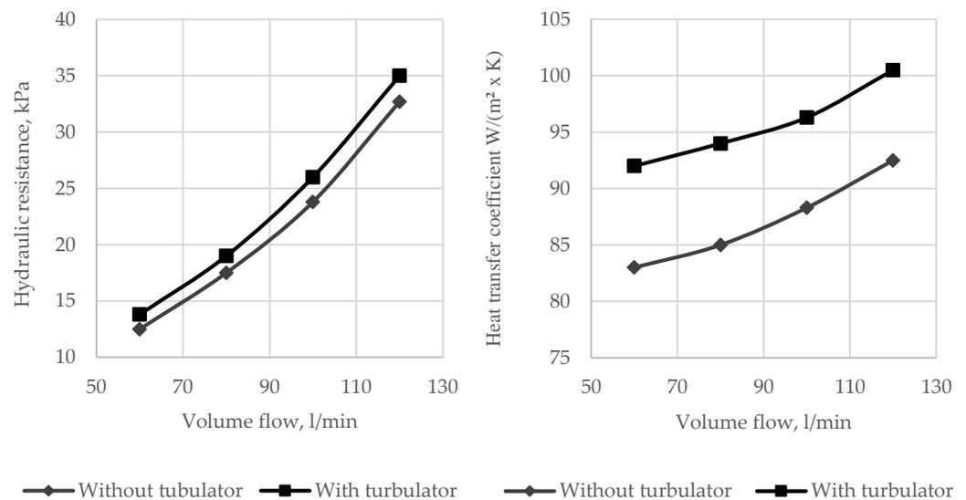
**Figure 1.** Plots of changes in hydraulic resistance and heat transfer coefficient depending on the flow rate of the working body for heat exchangers with and without turbulators.
