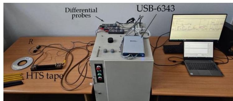
Figure 5. Laboratory test bench for recovery time.
