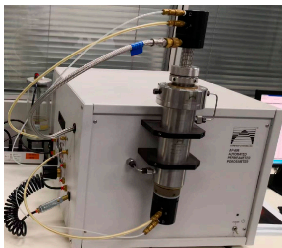
Figure 1. Experimental equipment used for porosity and permeability analysis.
