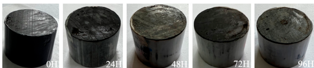
Figure 5. Shale core sample after \text{CH}_4 huff-and-puff.
