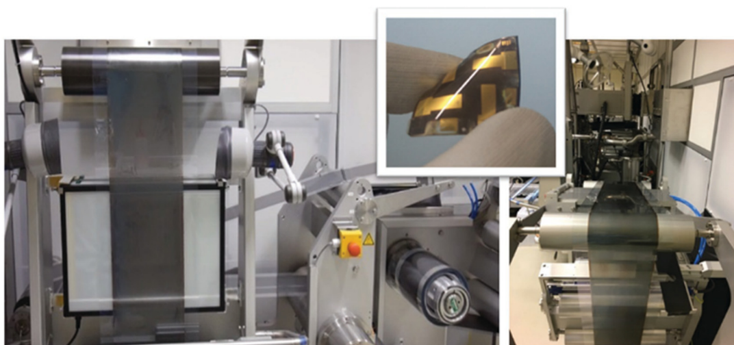
Figure 33. Pictures of the roll-to-roll deposition of the perovskite layer ( \text{Cs}_{0.15}\text{FA}_{0.85}\text{PbI}_{2.85}\text{Br}_{0.15} ), and an inset of a photograph of an example of the fabricated flexible device. Reproduced with permission from [109], John Wiley and Sons, 2018.
