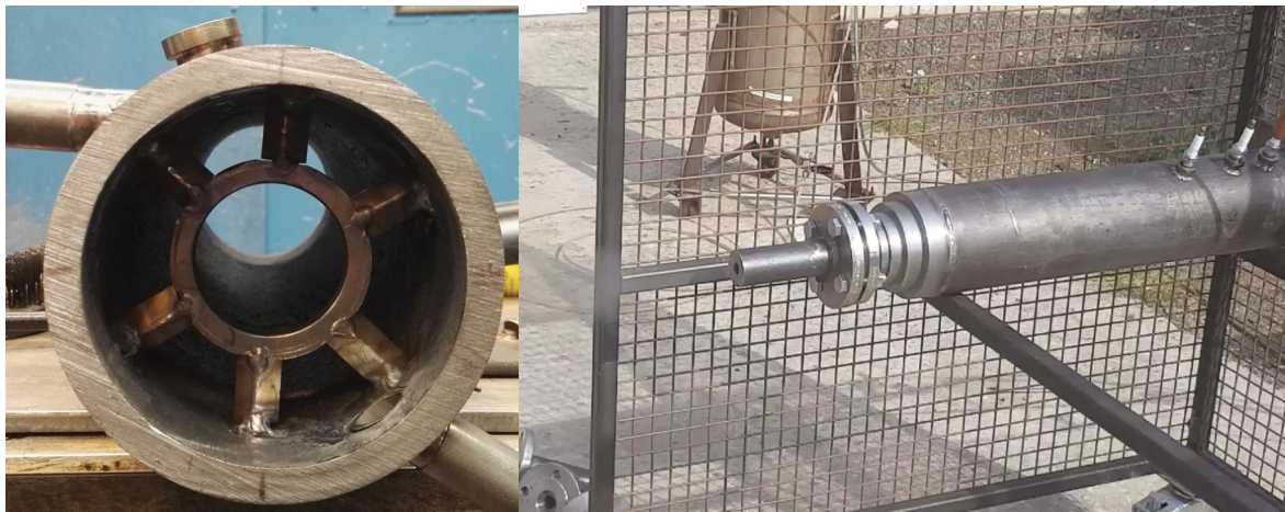
Figure 5. Manufactured high-pressure combustor.
