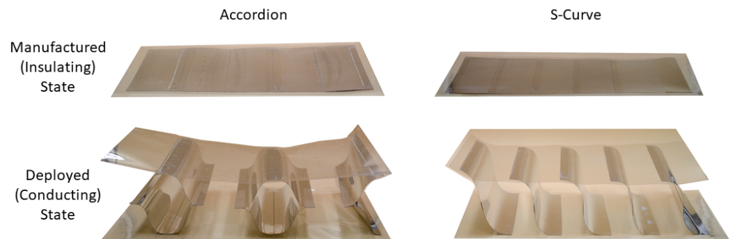
Figure 2. Two dynamic radiant barrier designs: Accordion fold and S-Curve. The DRBs in this image are made from polyethylene and metalized polyester.
