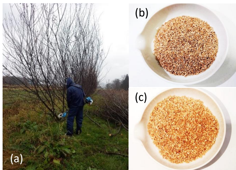
Figure 1. (a) Ezonokinu willow and its cuttings (5–6 cm diameter, ca. 1.1 dry-t/10 a) [30]; (b) crushed ezonokinu willow (with bark); (c) crushed cedar (without bark).
