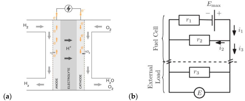
**Figure 1.** (a) PEMFC operation principle, (b) reduced order model scheme.
