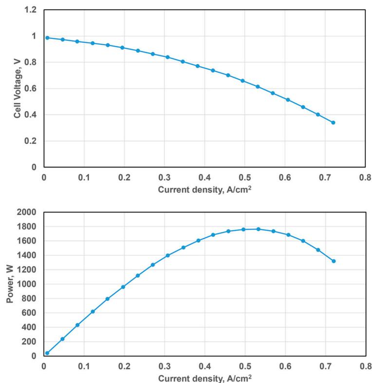
**Figure 4.** Simulation results of PEM fuel cell: current-voltage (**top**) and current-power (**bottom**) dependency.
