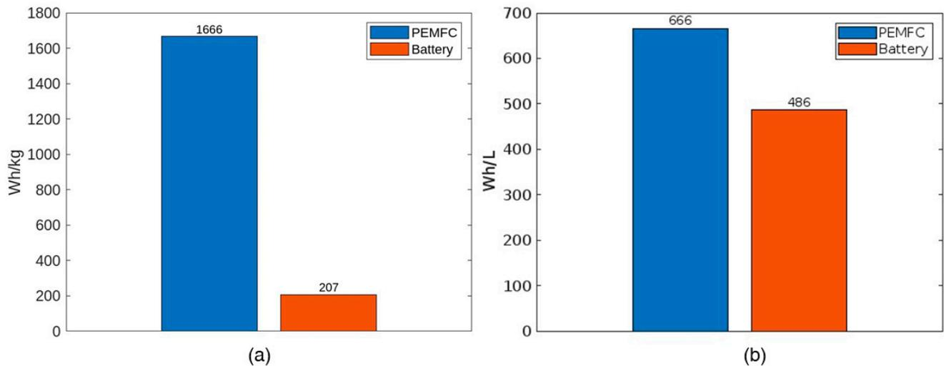
**Figure 5.** Specific energy of battery vs. fuel cell: (a) gravimetric; (b) volumetric.
