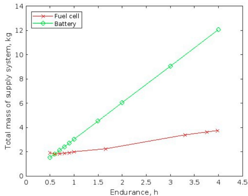
**Figure 6.** Total mass of the supply system vs. time of operation.
