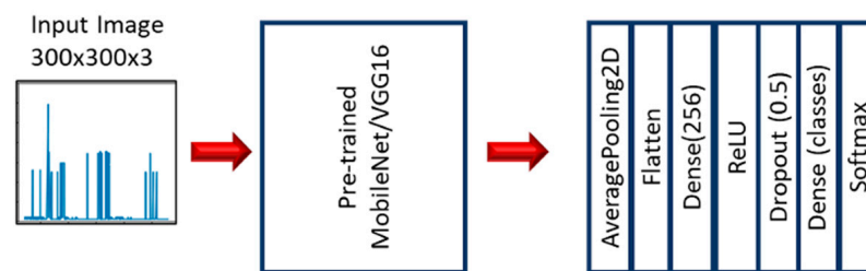
Figure 1. CNN architecture scheme Model 1.
