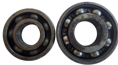
Figure 34. Bearings with defects 6203–2z/6204–2z.
