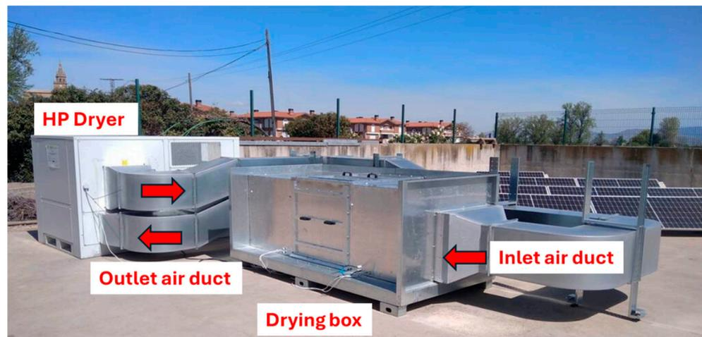
**Figure 2.** Drying infrastructure of the prototype of 2023. It consists of an HP dryer unit (which extracts humidity from the air), the inlet and outlet aluminum air ducts and the drying box (where the alfalfa bale is). The red arrows indicate the air flow direction.
