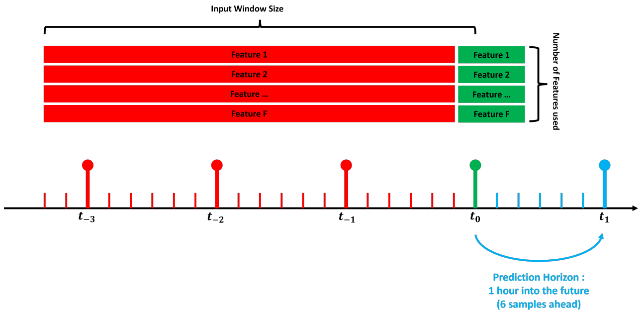
Figure 8. Illustration of the input to the prediction model, together with the prediction horizon. The input to the prediction model contains features in the past (red) and present (green). The prediction horizon defines a specific future time (blue stem) when the prediction is made.
