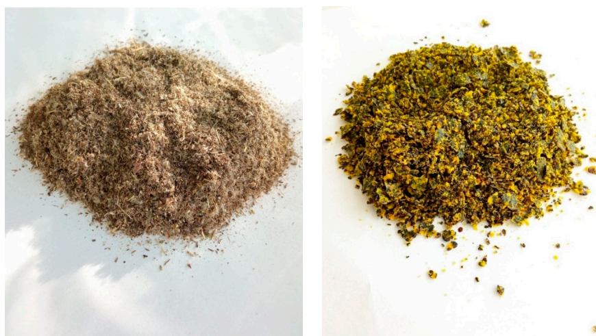
Figure 4. Prepared sorbents, from left : Canadian goldenrod (GB), right : rapeseed hulls (RHs).
