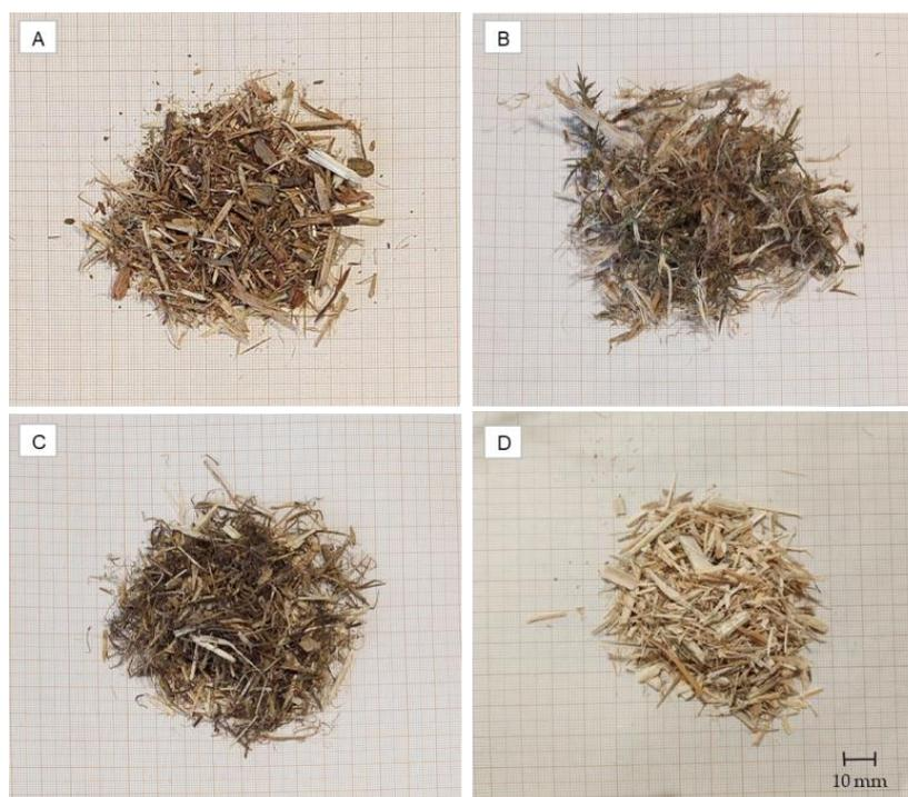
**Figure 3.** Macroscopic view of the biomass samples used in the pyrolysis experiments: (A) acacia, (B) gorse, (C) broom, and (D) giant reed.
